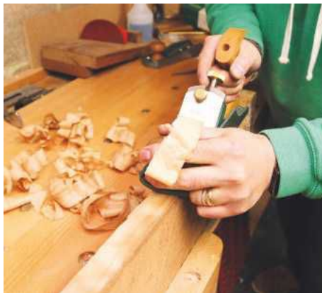
▲ There's a natural index finger resting point on the smoother but take care not to move the lever
